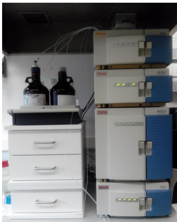
Figure 5 – ThermoScientific Accella Autosampler, Accella Pump 600 and Accella PDA detector
